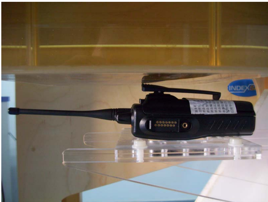
Fig.5 Test position_body Position (the EUT's antenna positioned 2.8cm from a flat phantom)
