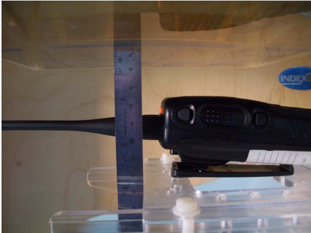
Fig.4 Test position_face Position (the EUT positioned 2.5cm from a flat phantom)
