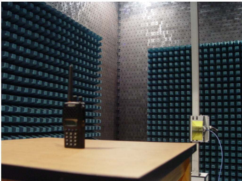
Photo 2 Radiated Emission Test
