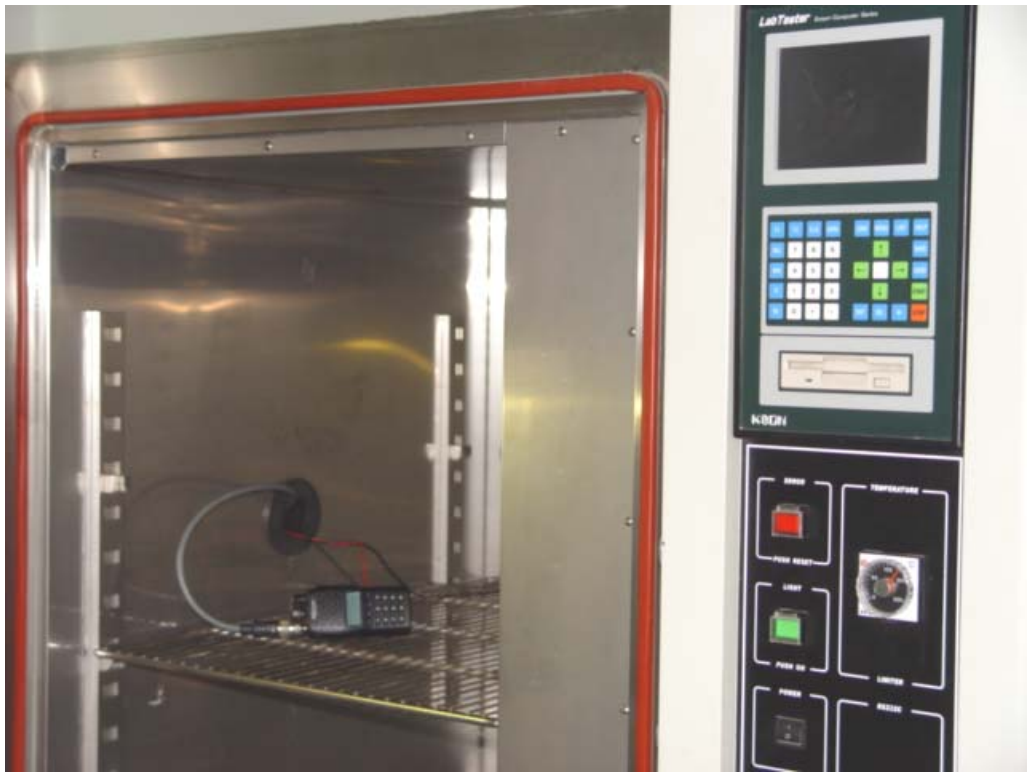
Photo 4 Transient frequency behavior Test
