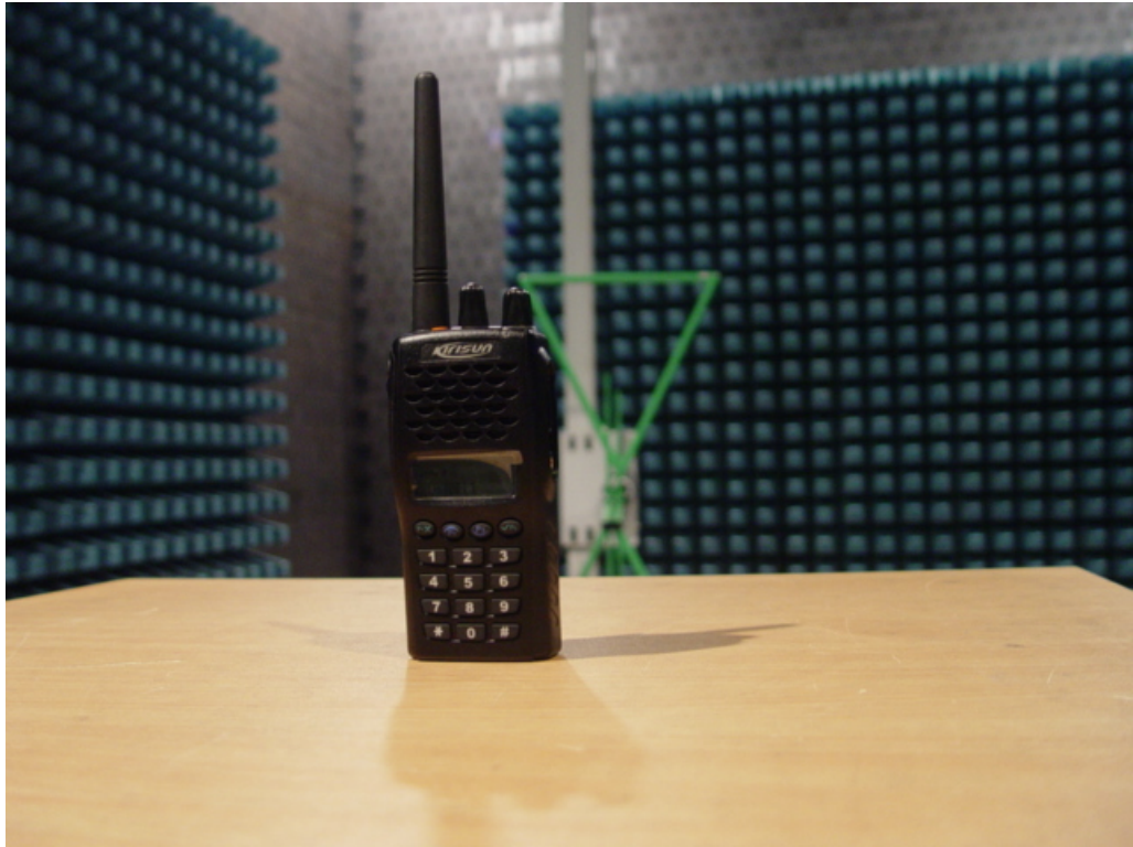
Photo 2 Radiated Emission Test
