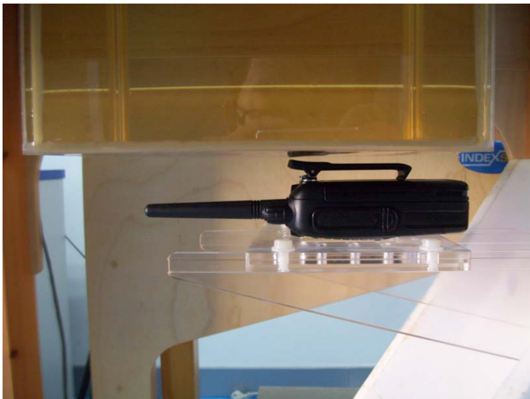
Fig.5 Test position_body Position (the EUT's antenna positioned 3.0cm from a flat phantom)
