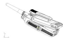
Press the lower end of the battery down until the latch of the radio completely bounces out, and the battery is locked.
