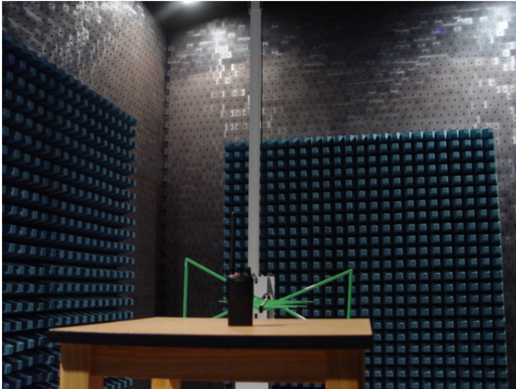
Photo 2 Radiated Emission Test
