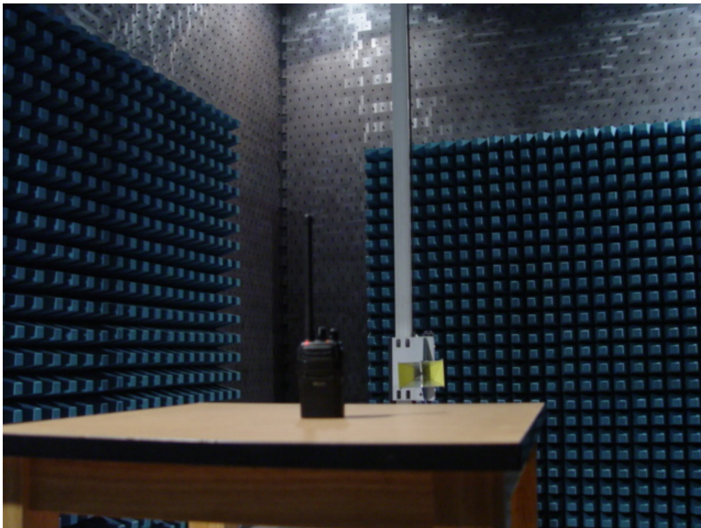
Photo 2 Radiated Emission Test
