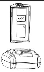
Insert the battery to be charged or the phone in the charger, please switch off the phone before installing it into the charger.
