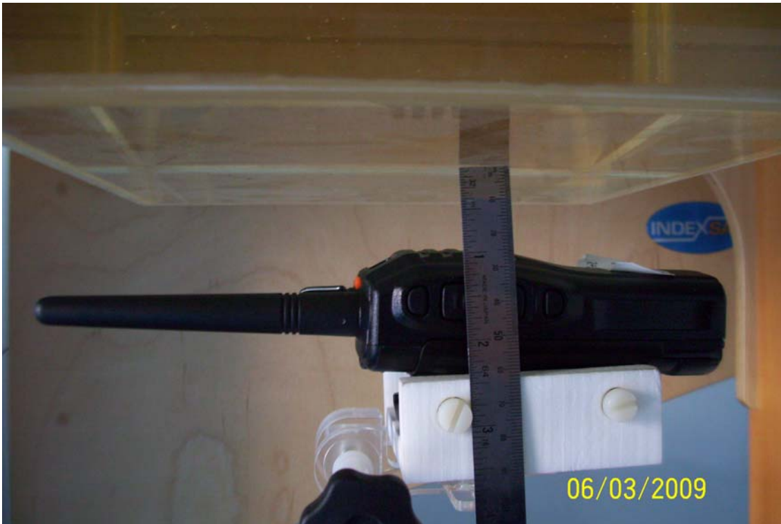
Fig.4 Test position_face Position (the EUT positioned 2.5cm from a flat phantom)
