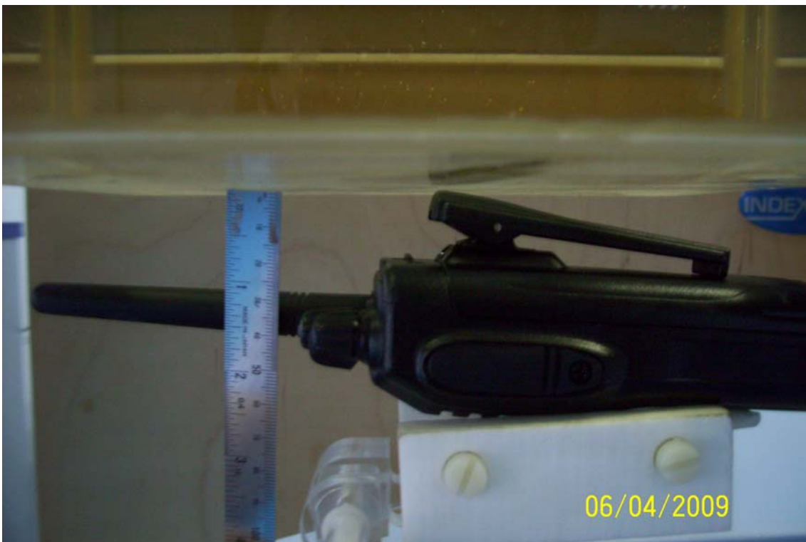
Fig.5 Test position_body Position (the EUT's antenna positioned 2.8cm from a flat phantom)
