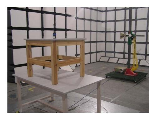
Radiated Emission - Rear View (Above 1000 MHz)
