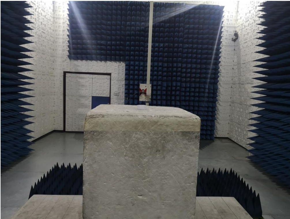
RADIATED EMISSION TEST SETUP ABOVE 1GHZ
