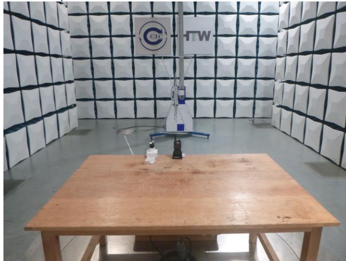
Radiated Emissions (30MHz-1GHz)
