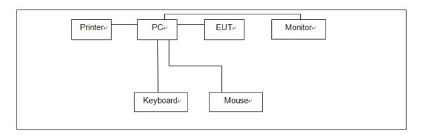
3.5. Support unit used in test configuration
