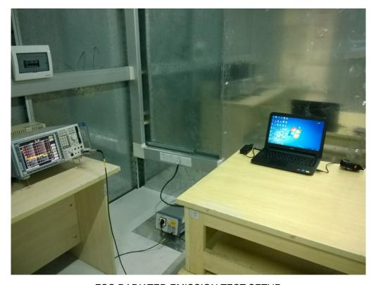
FCC RADIATED EMISSION TEST SETUP
