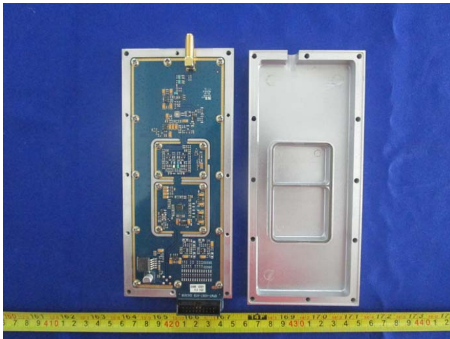
EUT – RX Board Cover Off View
