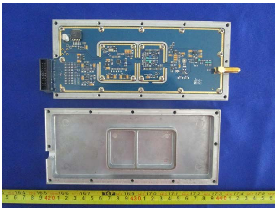
EUT – RX Board Cover Off View
