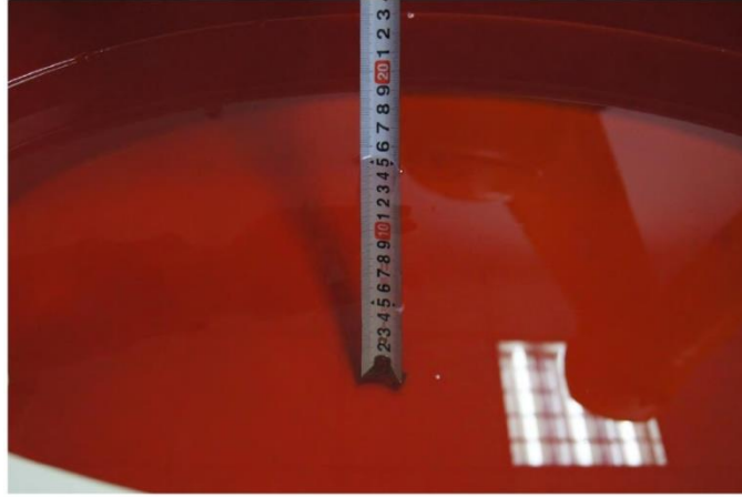
Liquid depth in the flat Phantom (450MHz) (15.3cm deep)
