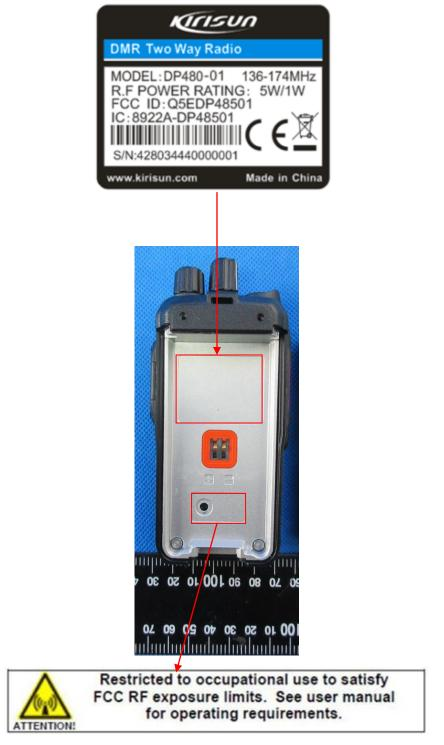
The label shown shall be permanently affixed at a conspicuous location on the device and be readily visible to the user at the time purchase (Labeling requirement per 2.925) Cover Model:
