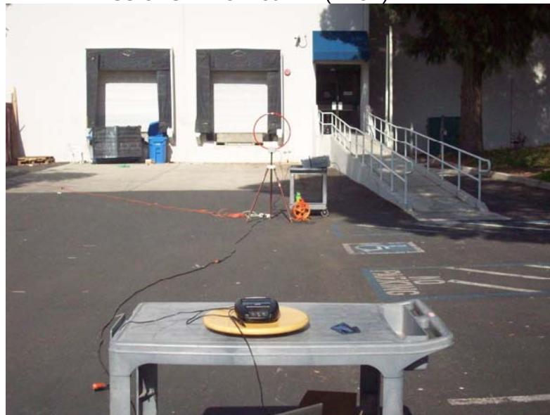
RADIATED EMISSIONS BELOW 30MHz (BACK)
