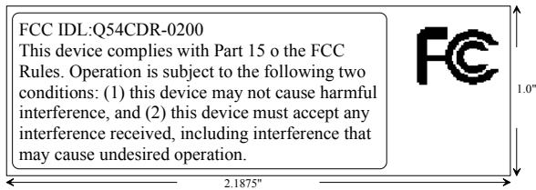
**Specifications:** Text is black in color and is left justified. Labels are printed in indelible ink on permanent adhesive backing and shall be affixed at a conspicuous location on the EUT.
