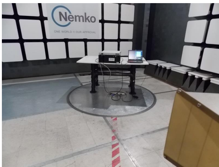
Figure 9.1-2: Radiated setup photo
