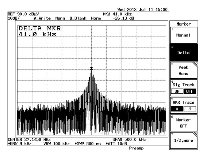
The field strength of any emission within the operation band did not exceed 80 dB(μV/m) for average value or 100 dB( $\mu$ V/m) for peak value.
