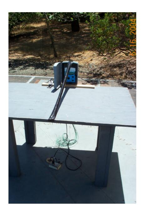
Rear View of EUT for Radiated Test, External Antenna (External antenna is taped to table to the right of the EUT, in this view.)
