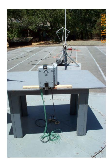
Front View of EUT for Radiated Test, External Antenna (External antenna is taped to table to the left of the EUT, in this view.)
