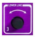
Knob #3 is the "LOWER LINE" control. One full turn of the knob clicks through 16 responses. There may be more than 16 possible responses, so just keep turning. If you go past the desired response, turn the knob the other way. At the end of a list of responses, further turning of the knob does nothing...it doesn't rotate around to the other end of the responses.
