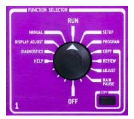
Knob #1, the "FUNCTION SELECTOR," will select which particular list is being viewed. Turn the knob in either direction. When you are done, don't worry about the knob position; the controller will irrigate in any position other than OFF.
