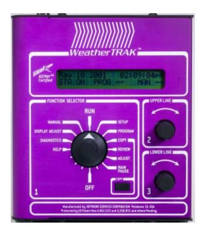
The underlying concept for the use of the *WeatherTRAK* controller is to visualize a series of lists that need to be filled out with information. What is seen in the display will change according to which list is being viewed. The Upper Line of the display identifies the information needed. The Lower Line of the display shows one of a selection of available responses. Three knobs are used to control the display.
