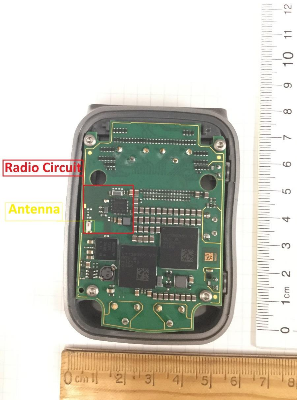
Figure 2: Wilson-I ETS Internal Photo – Frontside (radio circuit outlined)
