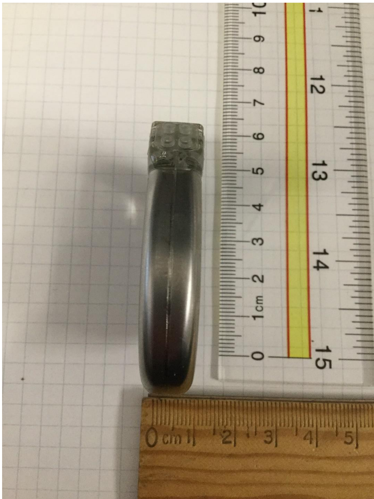
Figure 5: Wilson-I IPG External Photo – Header Ports
