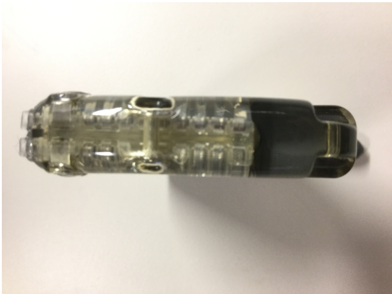
Figure 8: IPG External Photo of 2-Port Header of SC-1140/DB-1140
