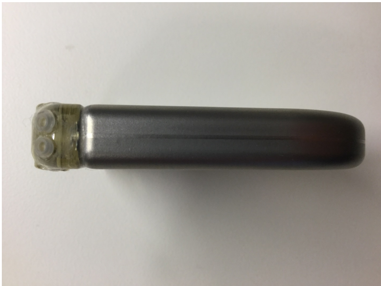
Figure 6: IPG External Photo of 2-Port Header of SC-1140/DB-1140
