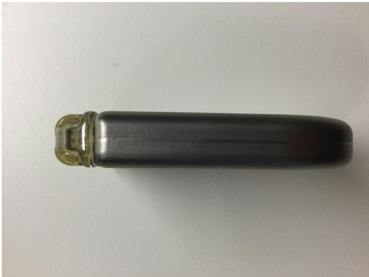
Figure 7: IPG External Photo of 2-Port Header of SC-1140/DB-1140
