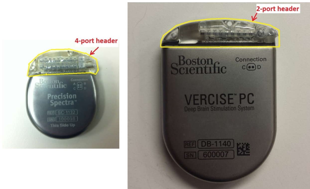
Figure 5: IPG External Photo, comparing SC-1132 (on the left) to DB-1140 (on the right), DB-1140/SC-1140 has larger enclosure case due to larger battery.
