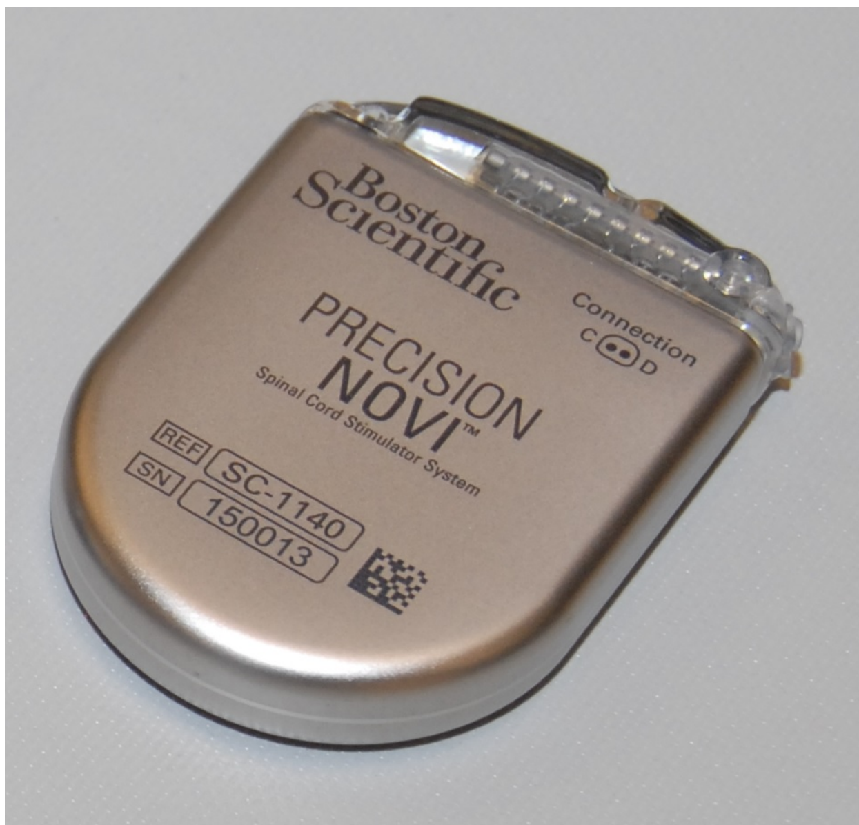
Figure 1: IPG (SC-1140) External Photo
