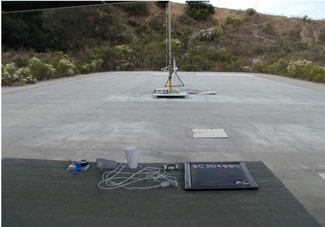
Photograph of Test Setup: Radiated Emissions
