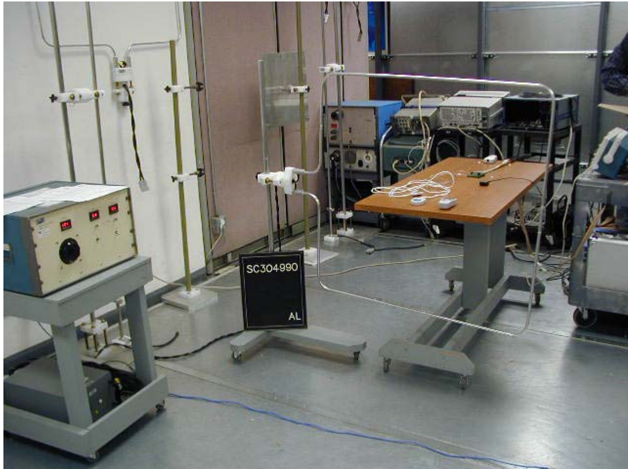
Photograph of Test Setup: Magnetic Field
