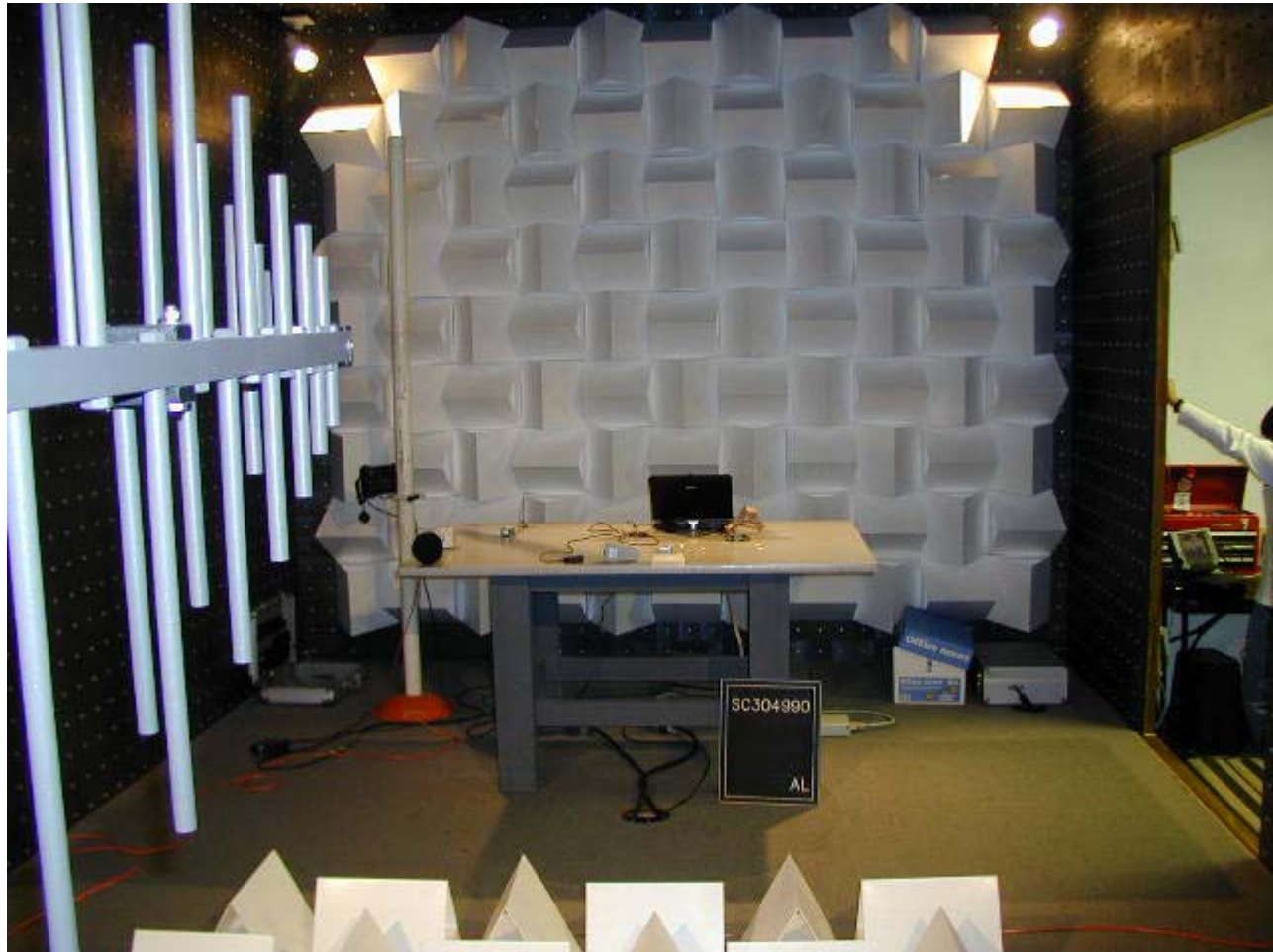
Photograph of Test Setup: Radiated Electromagnetic Fields
