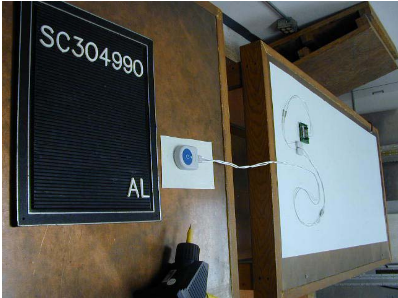
Photograph of Test Setup: Electrostatic Discharge (ESD)
