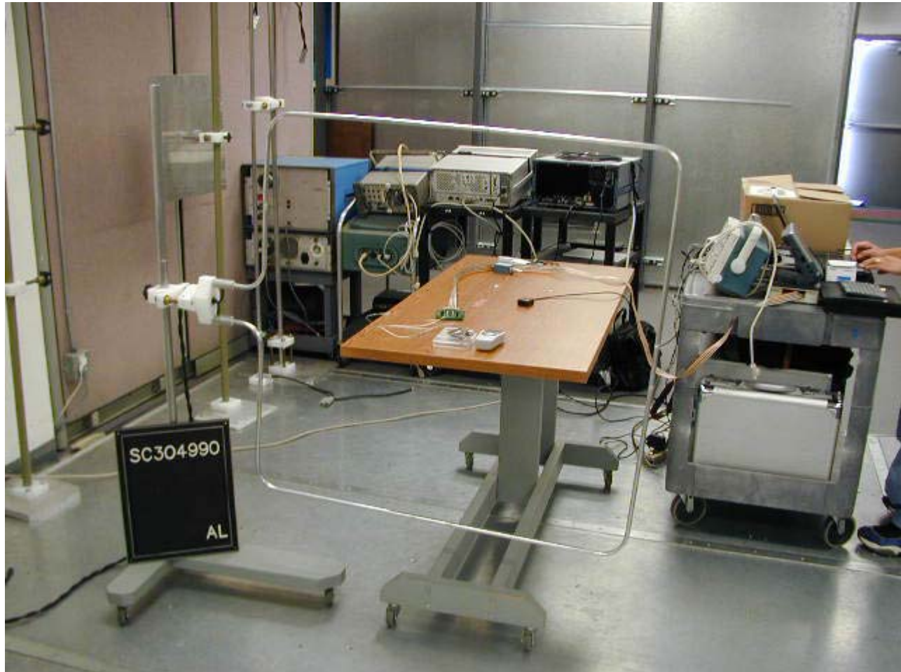
Photograph of Test Setup: Magnetic Field
