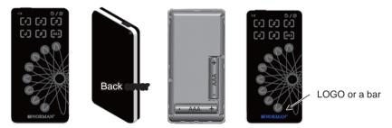
Turn over he remote and open the cover. Insert batteries (AAA batteries \* 2) matching the (+) and (-) marks and cover the bottom cover. If battery is assembled correctly, the LOGO will light on.
