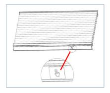
Press the button 3 times to enter Pairing mode. The green light will start flashing.
