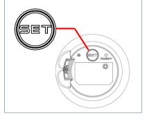
Hold SET for 3 seconds to enter Setup mode. The LED will start blinking.
