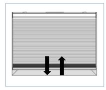
The shade will move up and down 2 times to indicate successful clearing.
