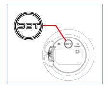
Hold SET for 3 seconds to leave Setup mode. The LED will stop blinking.
