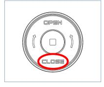
Press **CLOSE** to setup the Bottom position.
