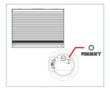
Hold RESET for 1 second. The Group LEDs will start blinking.
