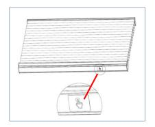
Press the button 3 times to enter Pairing mode. The green light will start flashing.
