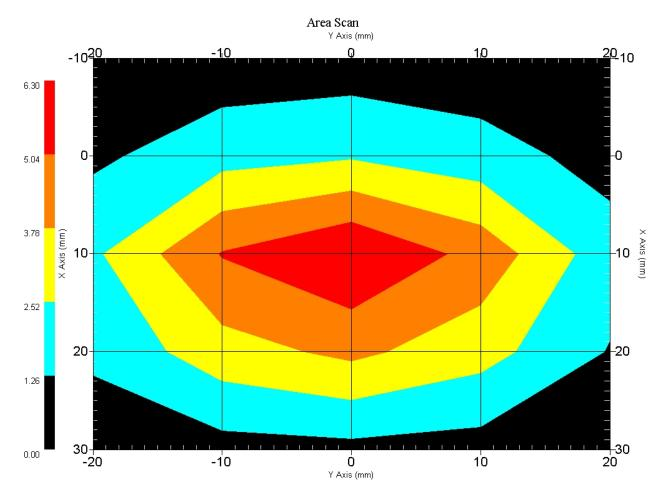
1 gram SAR value : 5.423 W/kg 10 gram SAR value : 2.488 W/kg Area Scan Peak SAR : 6.298 W/kg Zoom Scan Peak SAR : 11.090 W/kg
