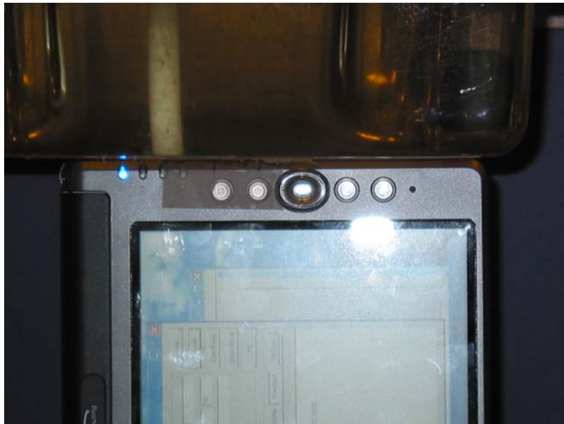
Main Antenna End Test Position Front View
