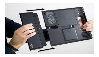
4. To remove the RFID Long Range Reader, insert your finger in the slot at the top of the reader, pull back the tab, and slide the reader off the Tablet PC.
