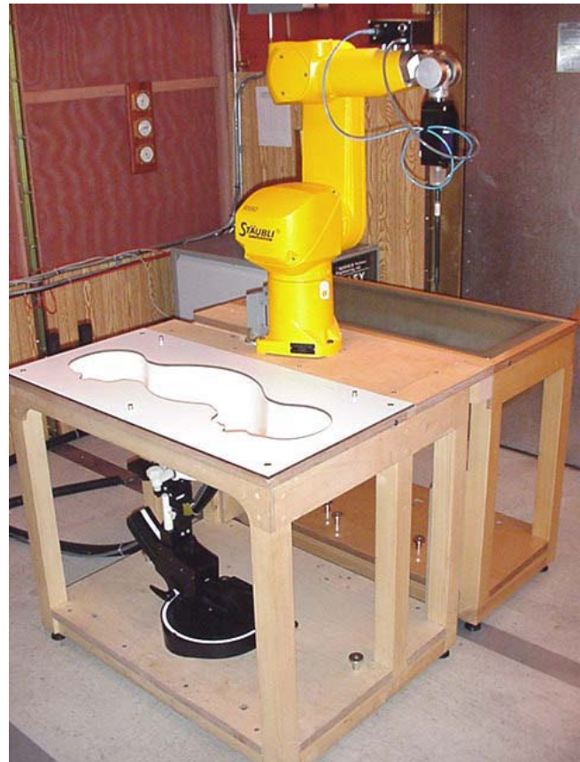
DASY4 SAR Measurement System with SAM phantom
