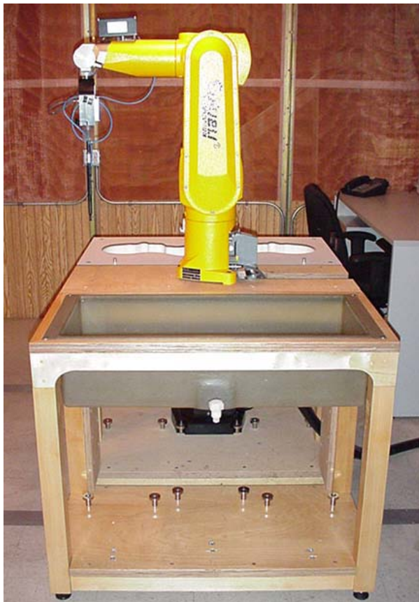
DASY4 SAR Measurement System with Planar phantom
