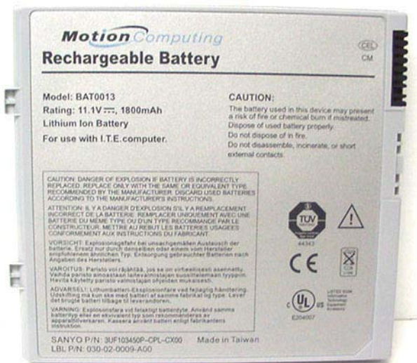
11.1V, 1800mAH Li-ion Battery Pack
