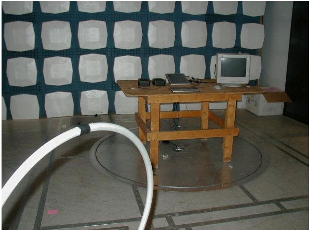
Photograph 1. FCC 15.209 Radiated Emissions Test Setup Photo
