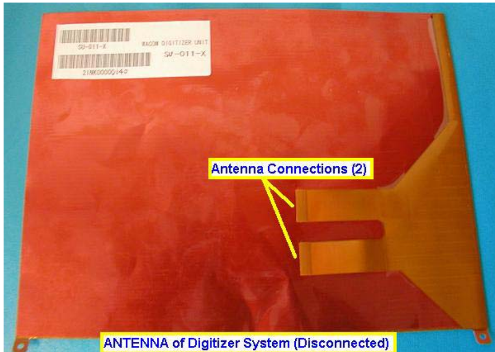
FIGURE 2: ANTENNA ALONE (DIGITIZER GRID)
