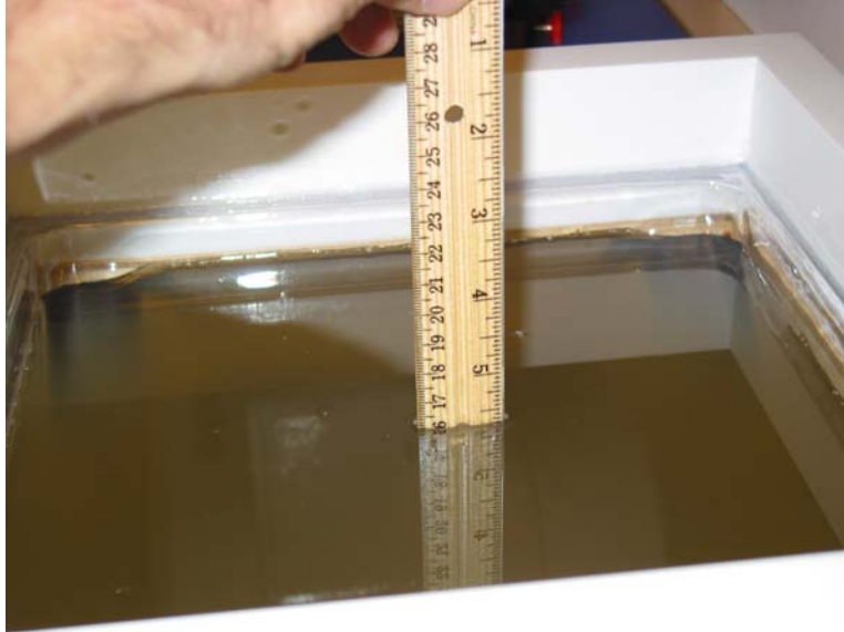
Figure 13 – Body Sugar Based Solution Tissue Depth
