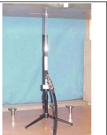
835 MHz Dipole Setup
