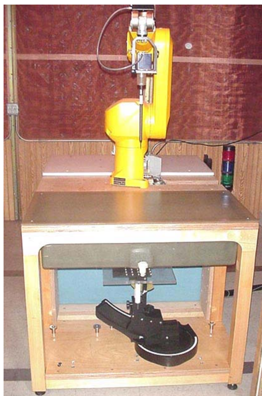
DASY4 SAR Measurement System with planar phantom
