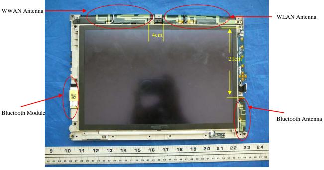
The co-located antenna between WLAN and WWAN is 4cm, the manufacturer has implemented software that selects only one of the WLAN or WWAN transmitters once a transmit function is invoked. So, There is no simultaneous transmission possible from the two transmitters, thus, simultaneous SAR testing is not required. Please refer the (Non-Simultaneous TX Statement.pdf) file for mode detail descriptions.
