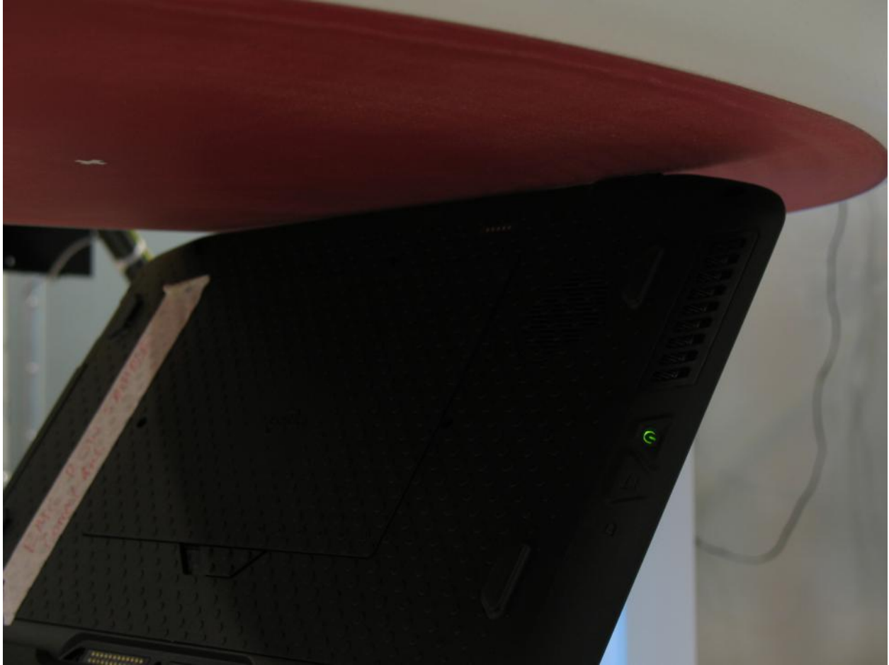
Figure 5: Device Positioning for SAR Scans – Top Edge Tilted 57 deg with no Spacing
