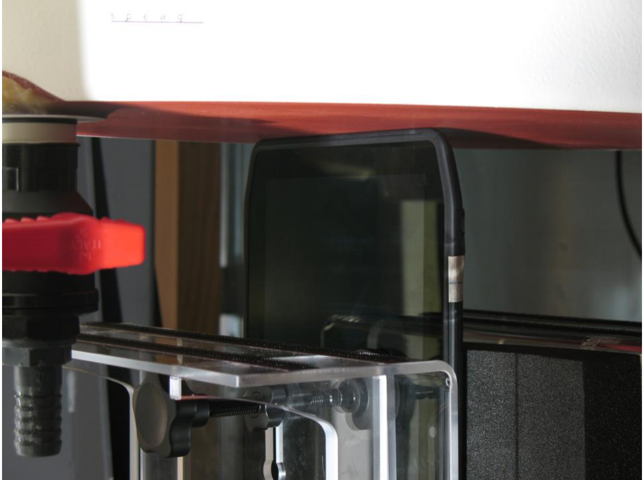
Figure 7: Device Positioning for SAR Scans – Left Edge Nearest WWAN Antennas with no Spacing
