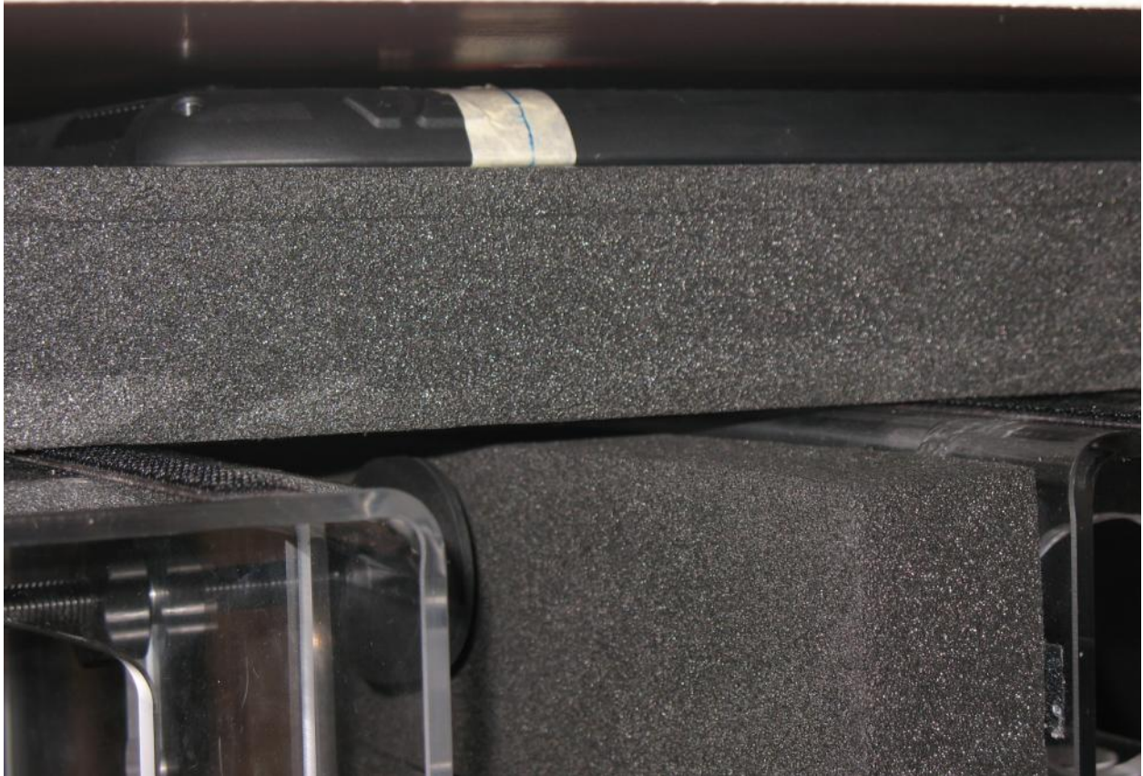
Figure 11: Device Positioning for SAR Scans - Back Against Phantom with 5mm Spacing
