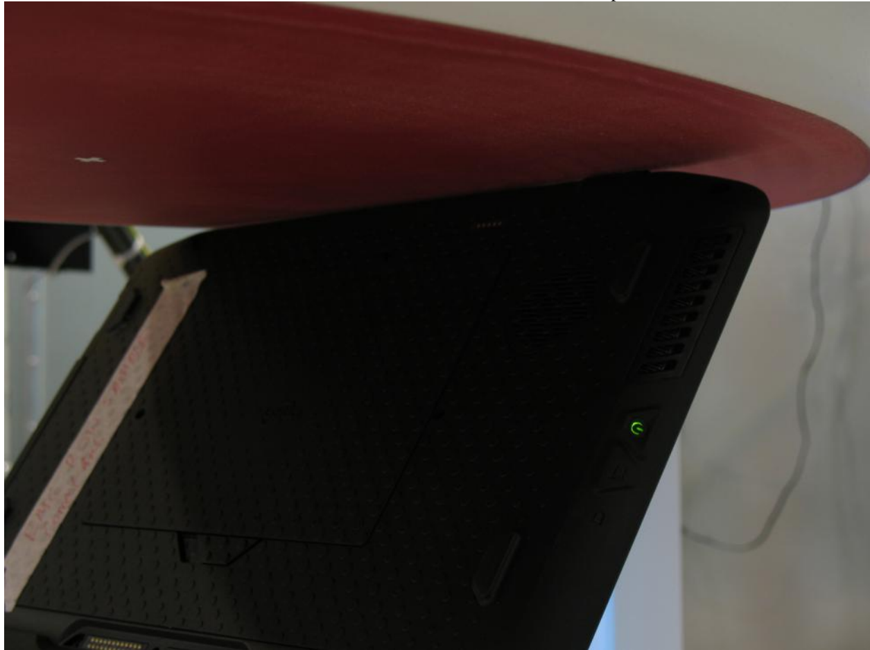
Figure 14: Device Positioning for SAR Scans – Top Edge Tilted 57 deg with no Spacing
