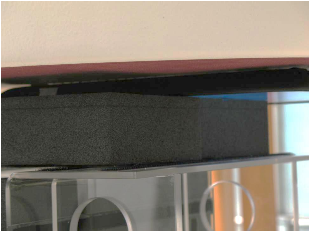
Figure 10: Device Positioning for SAR Scans – Back Against Phantom with No Spacing
