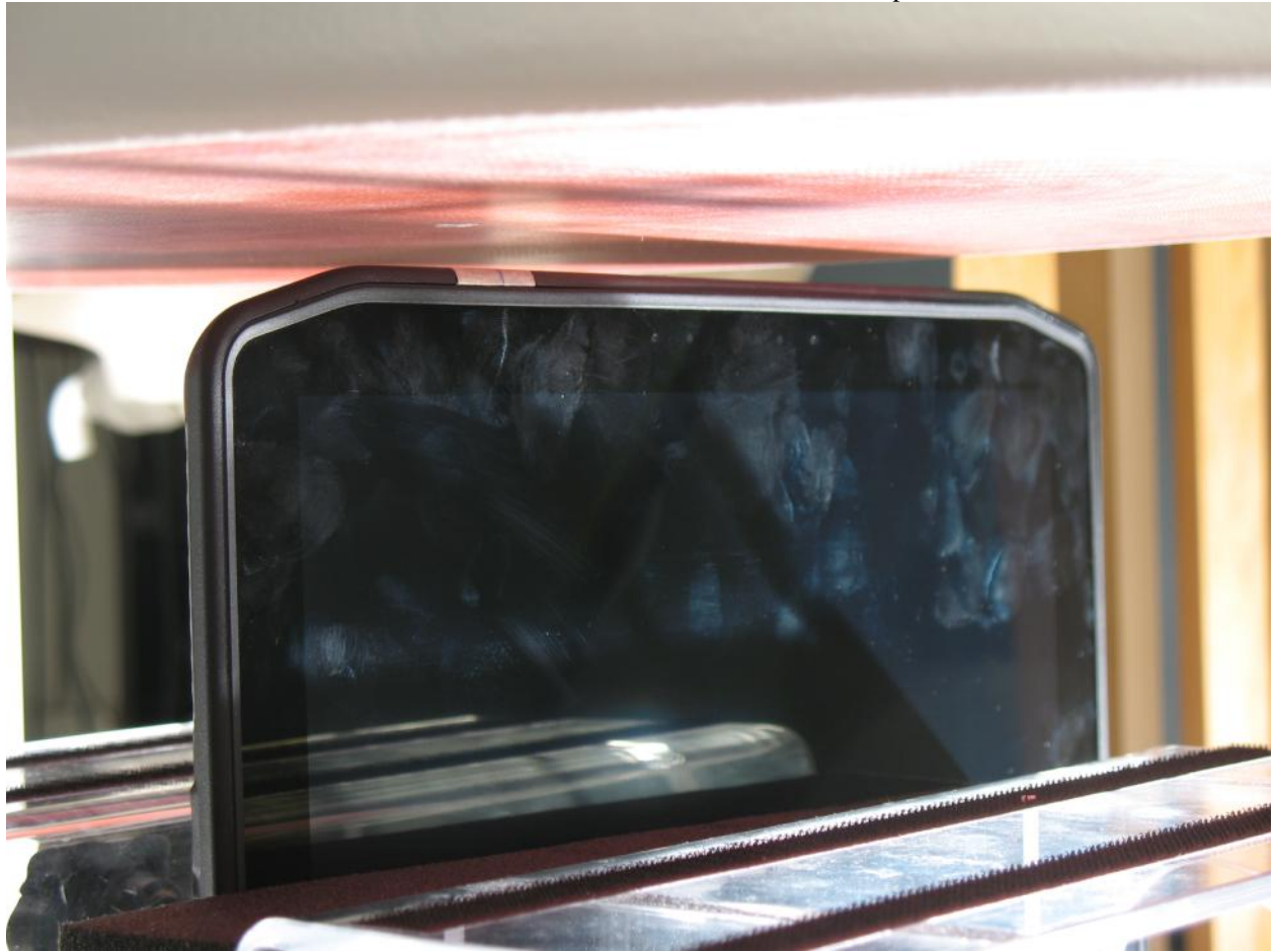
Figure 13: Device Positioning for SAR Scans – Top Edge with 9mm Spacing
