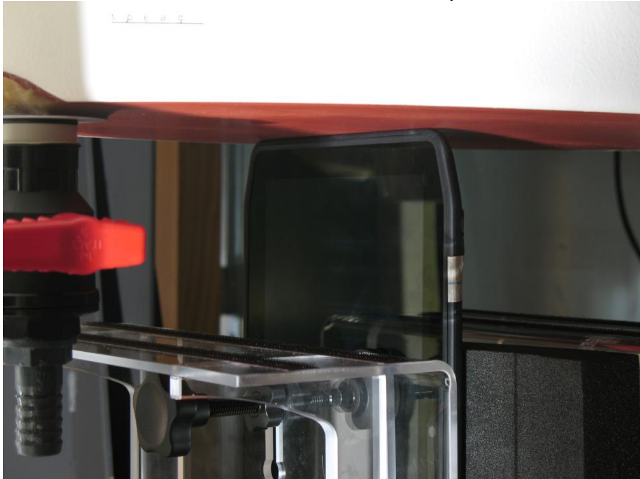
Figure 16: Device Positioning for SAR Scans – Left Edge Nearest WWAN Antennas with no Spacing
