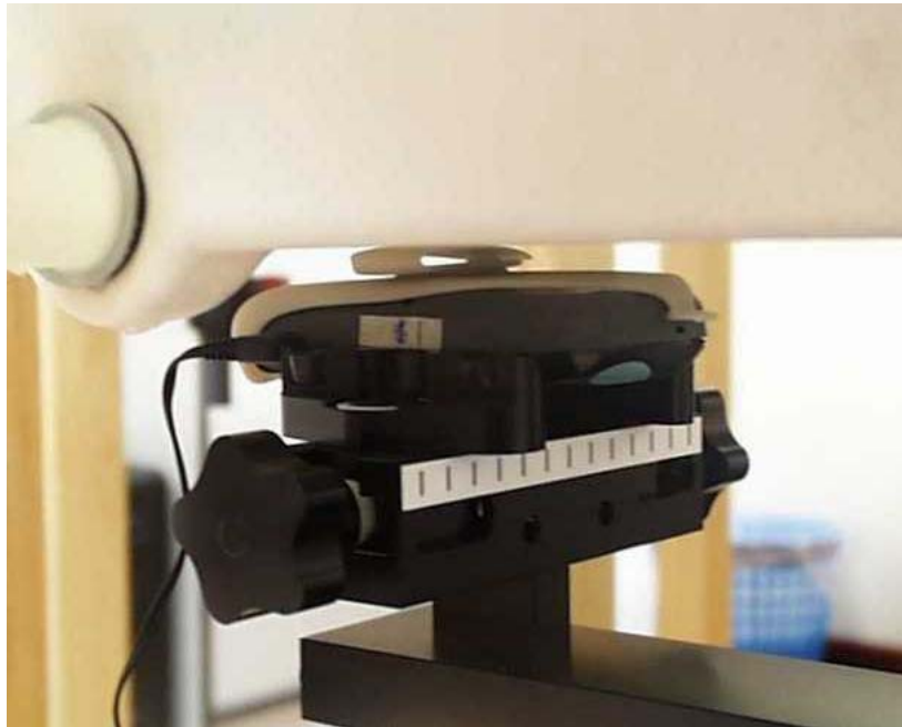
SAR Test Setup At Flat Phantom – Closer View (EUT Rear To Phantom)
