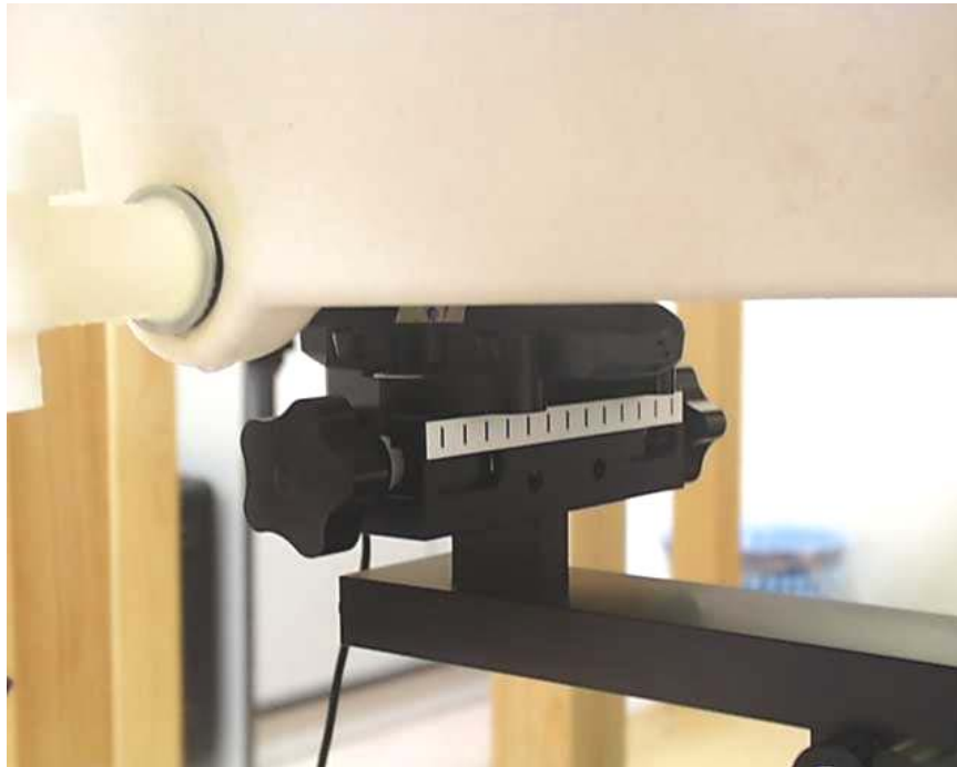
SAR Test Setup At Flat Phantom – Closer View (EUT Front Touched Phantom)
