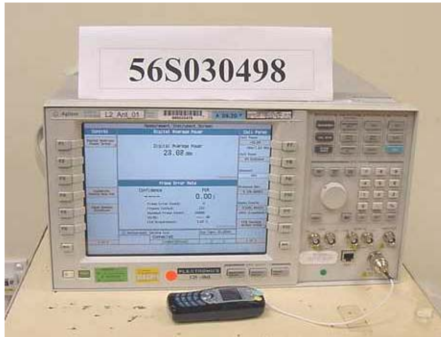
Conducted Power Measurement Test Setup
