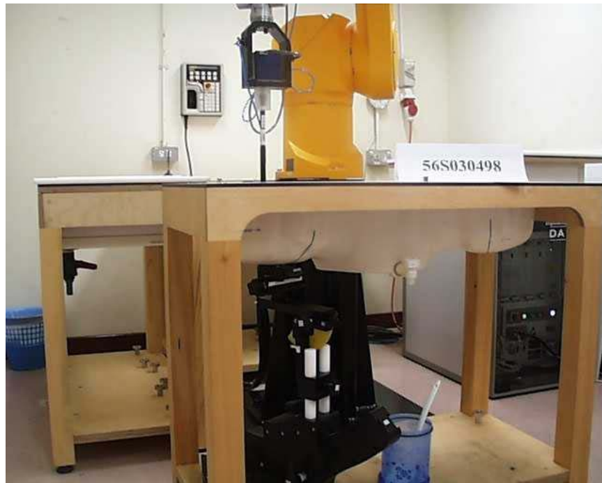
SAR Test Setup (Device at head phantom) – Far View
