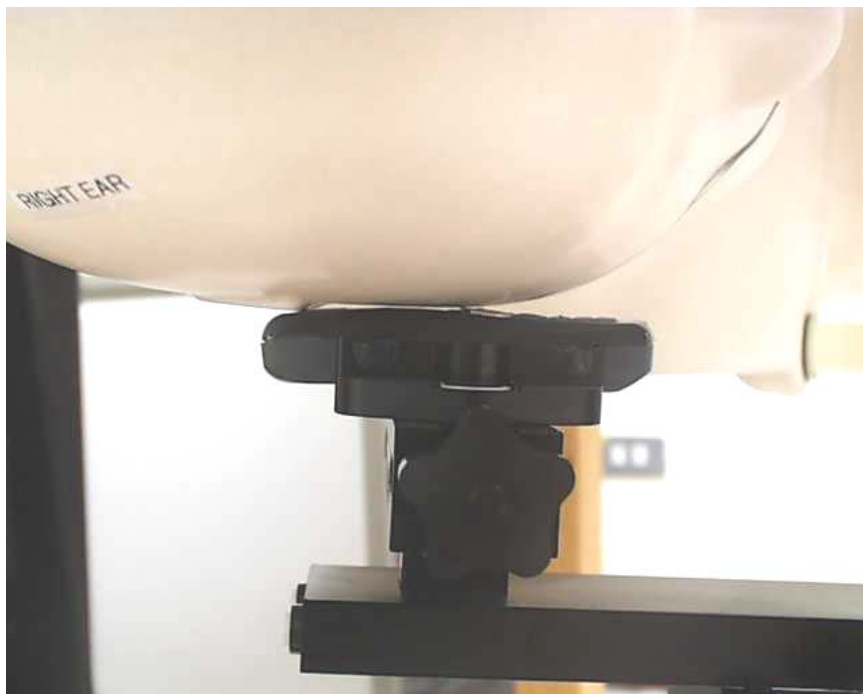
SAR Test Setup (Device at head phantom) – Closer Side View (Cheek/Touch)
