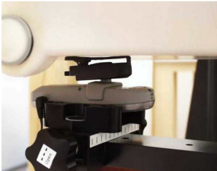
SAR Test Setup At Flat Phantom – View from Right Side (EUT Rear To Phantom, 26mm Gap Spacing)
