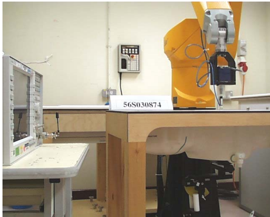
SAR Test Setup At Flat Phantom – Far View
