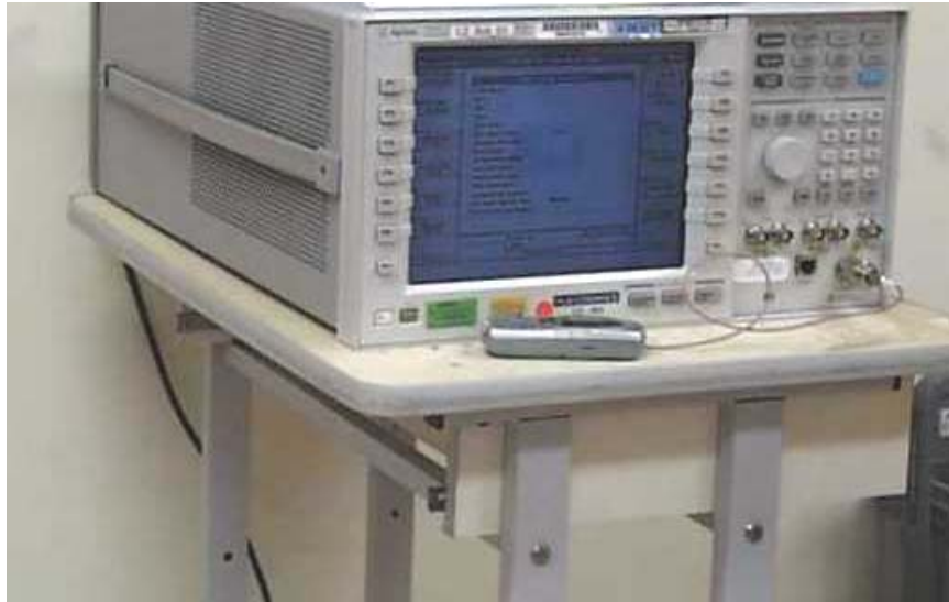
Conducted Power Measurement Setup
