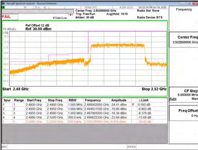
Bandedge B7 15M CH20825 QPSK(75,0)-FAIL VERIFY
