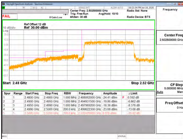
Bandedge B7 15M CH20825 QPSK(75,0)-FAIL
