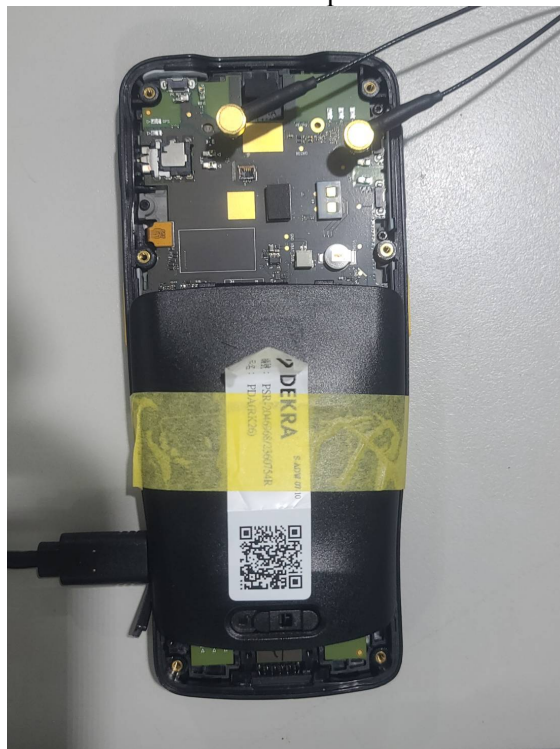
DFS Test Setup Photo
