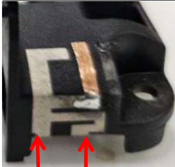
WiFi Main/Core0 antenna
