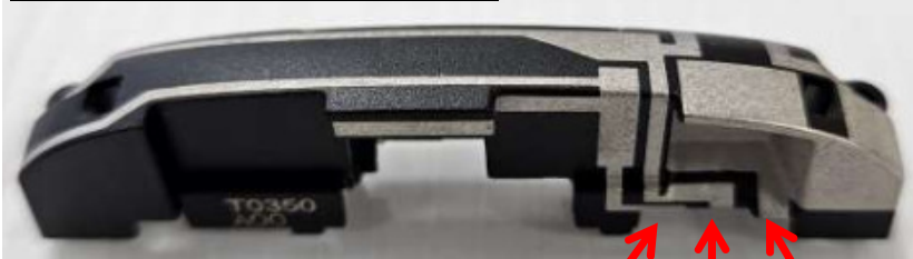
LTE Main antenna
