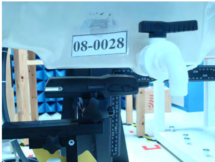
Figure 17. Body SAR Test Setup (Flat Section) _ 13 mm separation
