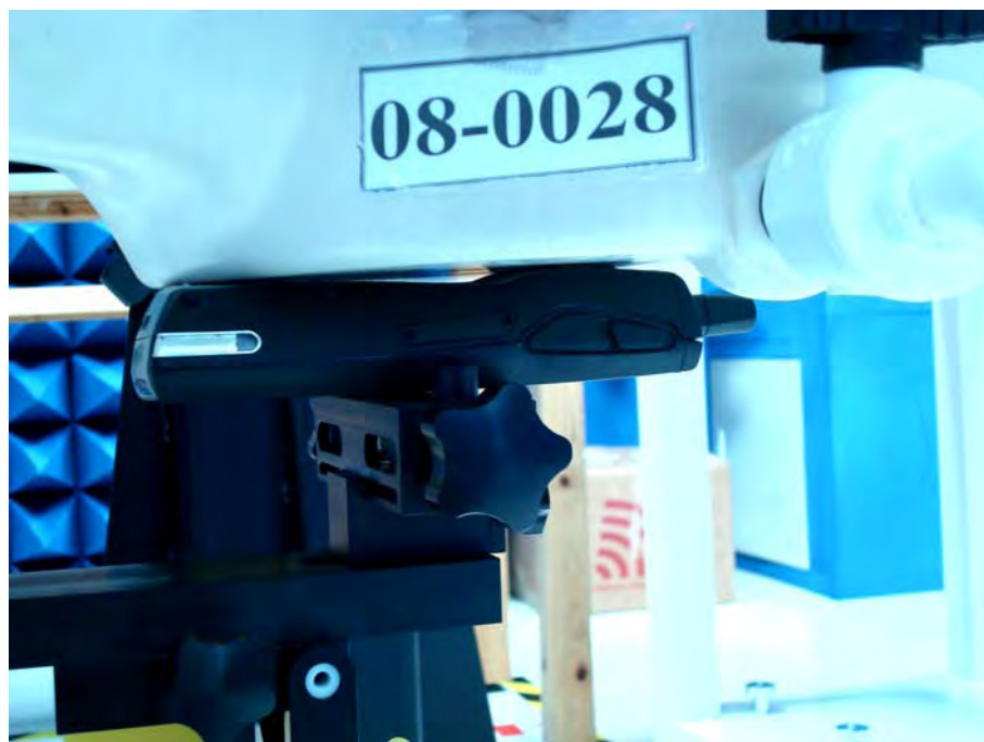
Figure 18. Body SAR Test Setup (Flat Section) _ 0 mm separation
