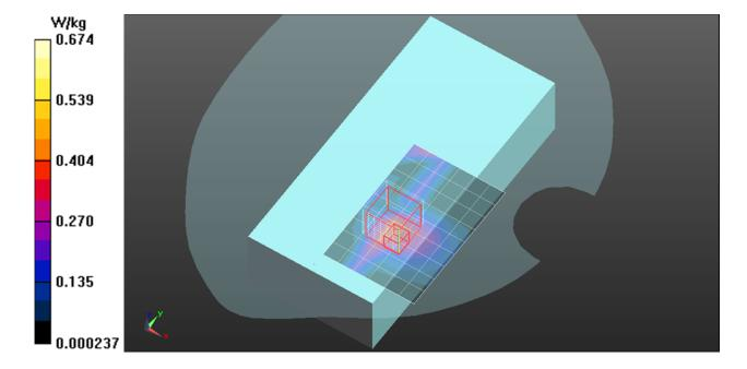
Frequency: 5560 MHz; Duty Cycle: 1:1; Room Ambient Temperature: 24.5°C; Liquid Temperature: 24.0°C Medium parameters used: f = 5560.9 MHz;  $\sigma = 5.557$  S/m;  $\epsilon_r = 48.21$ ;  $\rho = 1000$  kg/m<sup>3</sup> DASY5 Configuration:
