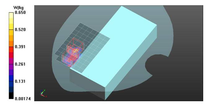
Frequency: 5520 MHz; Duty Cycle: 1:1; Room Ambient Temperature: 24.5°C; Liquid Temperature: 24.0°C Medium parameters used (interpolated): f = 5520 MHz;  $\sigma = 5.52$  S/m;  $\epsilon_r = 48.317$ ;  $\rho = 1000$  kg/m<sup>3</sup> DASY5 Configuration:
