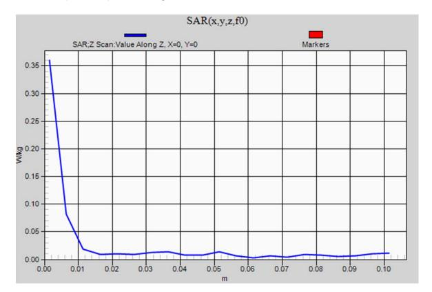
Frequency: 5680 MHz; Duty Cycle: 1:1; Room Ambient Temperature: 24.5°C; Liquid Temperature: 24.0°C Medium parameters used (interpolated): f = 5680 MHz;  $\sigma = 5.7$  S/m;  $\epsilon_r = 48.051$ ;  $\rho = 1000$  kg/m<sup>3</sup> DASY5 Configuration:
