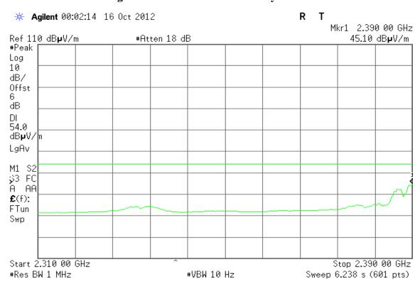
Detector mode: Peak Polarity: Horizontal
