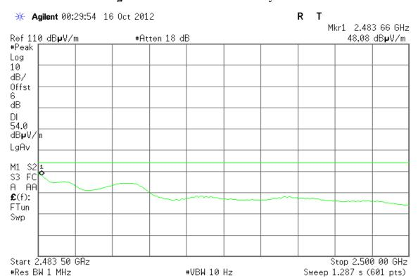
Detector mode: Peak Polarity: Horizontal
