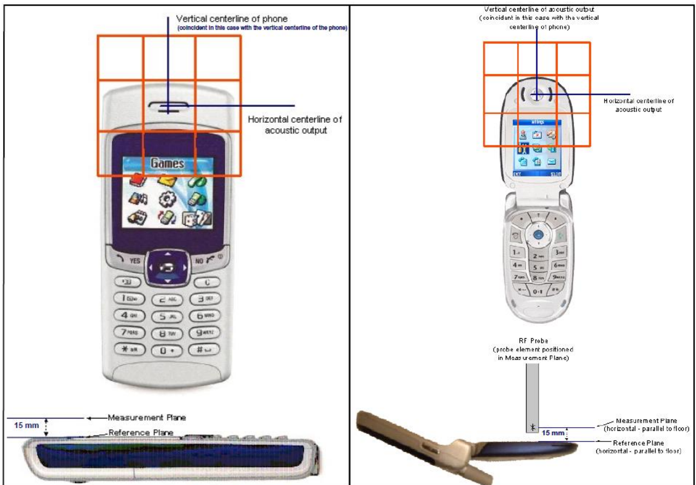
Fig-3.5 EUT Reference and Plane
