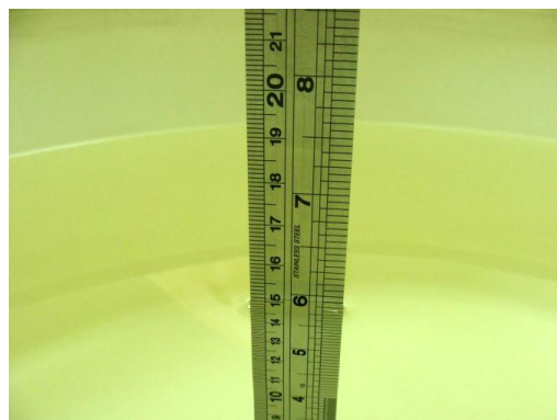
Fig 6.2 Photo of Liquid Height for Body SAR
