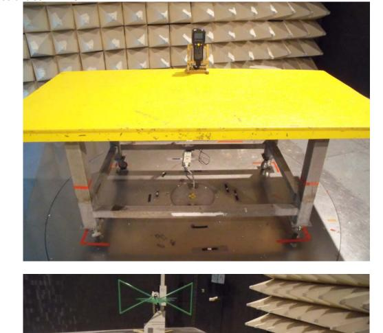
For radiated emissions 30MHz~1GHz
